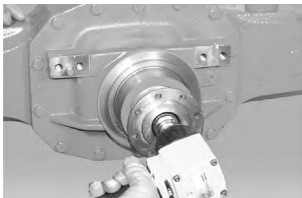
Position tool, so as to avoid pinion rotation. Unloose and remove the nut (1).
