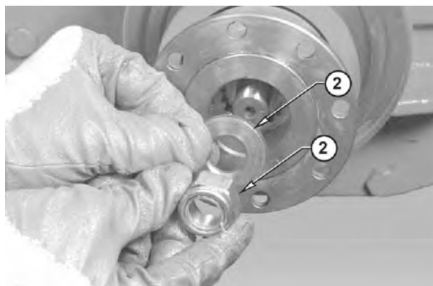
Unloose and remove the nut (1); also remove the washer (2) and (2) and shims (3).
