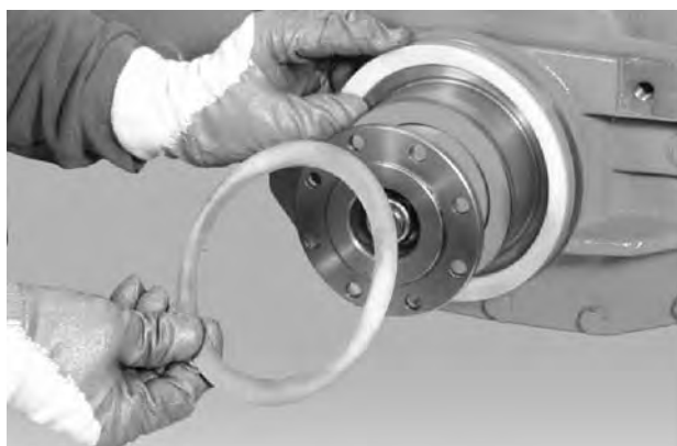
Remove the bottom front sealing ring and shims.
