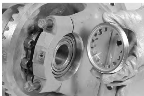
Mark the position of the ring nut (24) and differential support (13).
