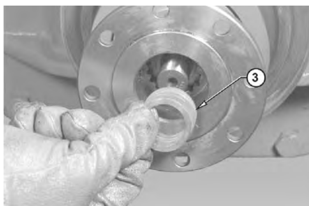
Unloose and remove the nut (1); also remove the washer (2) and (2) and shims (3).
