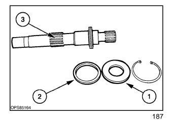
11. The motor shaft, thrust bearing assembly, consists of two retaining rings, 1, two thrust washers,2, and a thrust bearing,3. Disassemble these parts for inspection.
