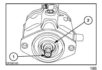
10. Remove the outer shaft seal, 1, and washer, 2, from the motor drive shaft, 3.
