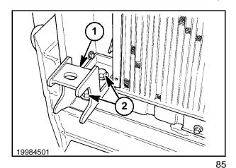
10. Remove eight mounting cap screws, 1, (four screws on each side). Remove the radiator/oil cooler assembly from the skid steer.
