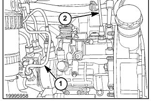
8. Loosen clamps, 1, and remove the fuel tank filler neck, 2.
