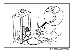
2. Inspection of protrusion at cylinder liner flange
