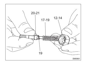
Push spring seat 1 (12) so that the movement is 7 mm or less, and install spool (20) through the large hole of spring seat 1.
