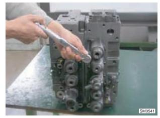
2.2 Draw out the assy of travel spool (306), spring seat (331), springs (323), (324), stopper (336) and bolt (333) from casing A (101) or casing B (102).
