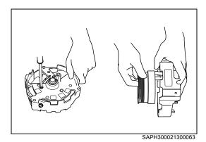
Remove five bolts using a screwdriver and remove the heat sink assembly (plus), heat sink assembly (minus) and regulator all together.
