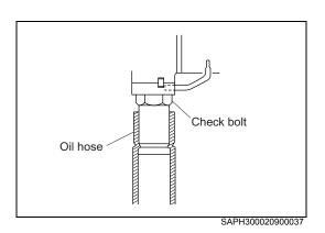
(2) Connect the injection test oil hose from the lower part of the cylinder block to the special tool check bolt.
