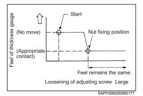
(5) Loosen the adjusting screw of the crosshead with the thickness gauge inserted. Make sure that feel on the thickness gauge is not lighter.
