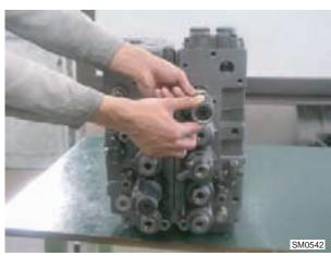
2.3 Fix the travel spool assy with vise via a protective plate (aluminum plate, etc.). Remove bolt (333) and separate spring seat (331), springs (323), (324) and stopper (336) from travel spool (306).
