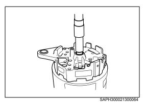
Remove the roller bearing from the rear bracket using a press, jig A and jig B.
