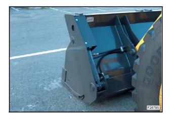
Unscrew and remove the clamping screws of the cover (C).
