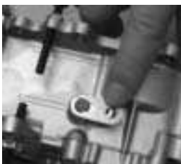
Remove the removal stop, (governor lever shaft).
