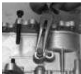
Pull out the governor lever shaft.
