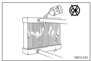
**Caution:** The cooling water passages in the engine must be completely filled with cooling water.
