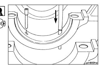
Make sure that the spray hole is clean and not clogged.
