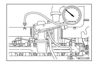
If the resistance exceeds the specification, check the oxidizing catalyst and/or muffler, and replace.
