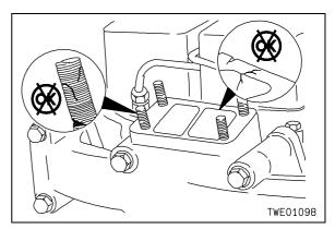
**Caution:** If you are not going to replace the turbocharger immediately, block the opening to prevent dust from entering the manifold.
