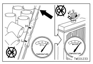
The cooling system is designed so that the specified amount of cooling water is used. If the water level is low, the engine will operate at a temperature higher than the specified temperature.
