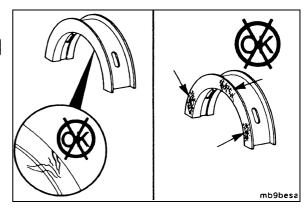
Measure the thickness of the flange of each thrust bearing. Measure the contact areas on front and rear sides.
