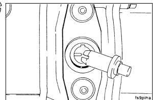
★ Install the fuel injection pump O-ring. Check that the position of the O-ring is correct and that it is not damaged.
