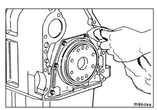
★ The center bolt hole on the flywheel housing mounting pad passes right through. Coat the stop screw with Loctite 277 and install it in the hole.
