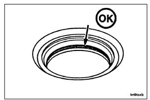
Set the cutter motor so that the cutting tool will cut only the valve seat insert and will not enter the machined valve pocket of the cylinder head.
