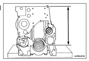
Check the main bearing holes for wear and damage. Install new main bearings and tighten the main caps, then measure the diameters of the holes.
