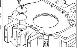
Clean the flywheel housing and cylinder block mounting surfaces completely. Wash these surfaces. There must be no oil or accumulated dirt on them.
