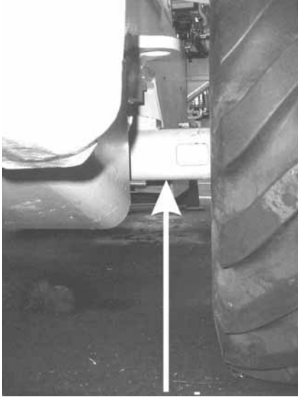
Fig. 15.3. Rear Axle Machine Support Point
