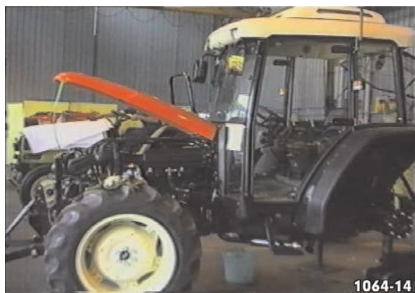
Fig. 15 - Disconnecting the parts connecting the cab to the tractor.
