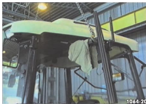
Fig. 16 - Lifting the cab off the tractor using a hoisting.
