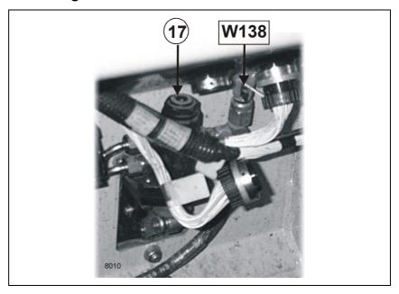
W138 Pressure switch for the brake lights17 Kicker plate brake valve
