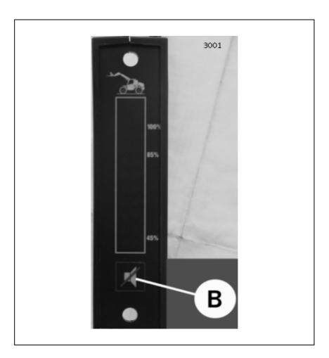
B This button is to test the load indicator and to mute the warning buzzer.
