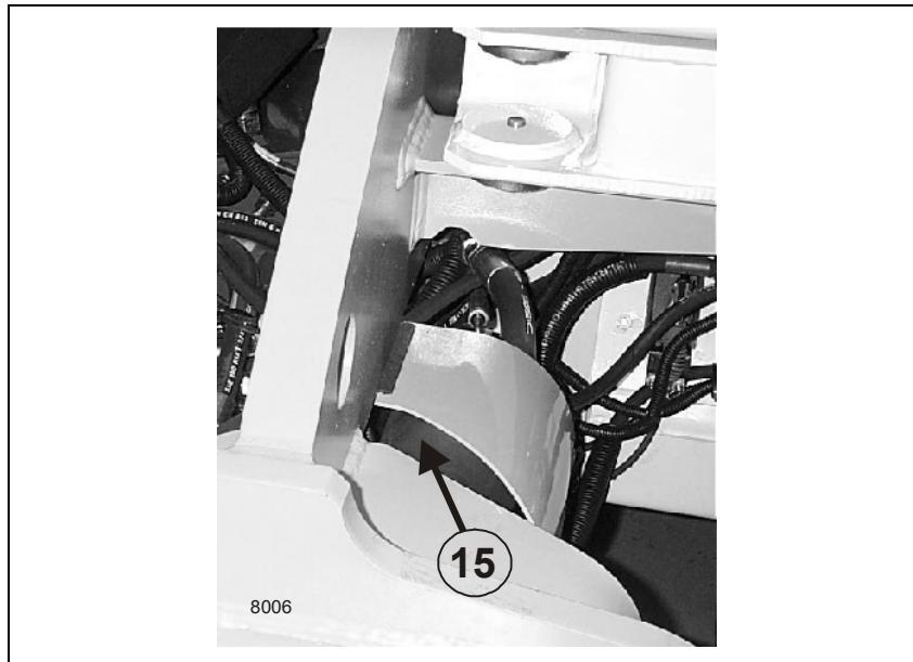
15 Accumulator pre-tensioned to 41 bar
