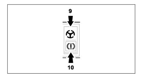
Warning light steering pressureWarning light brake pressure
