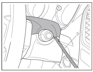
Prise open along the steering column upper and lower shields with the interior trim removal tool (BF1102) [1], and remove the steering column upper shield (1).
