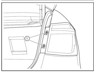
Remove 2 fixing screws (1) of the fixed side tail lamp with a Phillips screwdriver.
