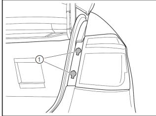
Pry up the 2 screw covers (1) of the fixed side tail lamp with a slotted screwdriver.
