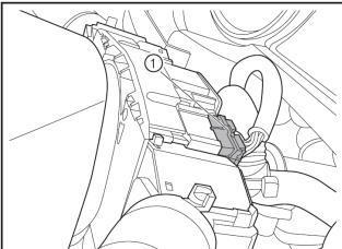
Disconnect the connector (1) of wiper combination switch.
