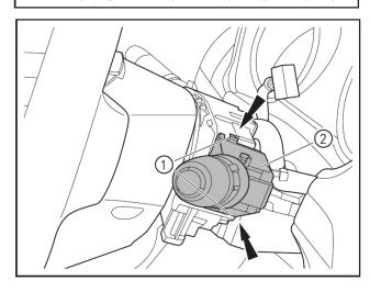
Press the clip (1) as directed by the arrow, and remove the wiper combination switch (2).
