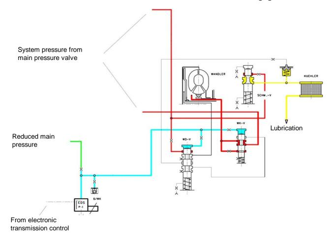
Vhen overlap gear shifts take place, freewheels are not used but are replaced by suitable actuation of the relevant clutches (electronic-hydraulically). This enables both weight and space to be saved. The electronic-hydraulic shift action is obtained by means of various valves in the hydraulic control unit,
