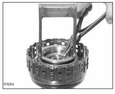
Using installation bracket 5x46 001 499, press the baffle plate down and remove snap ring with suitable pliers. Take out baffle plate and cup spring and remove O-ring from baffle plate.
