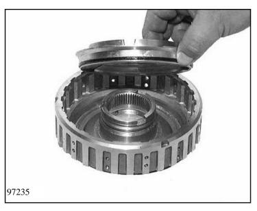
Install new O-rings 75.010/130 and 75.010/140 on piston C 75.010/120. Press piston into cylinder C 75.010/110.
