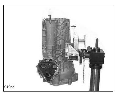
Place measuring element in transmission housing on the bearing contact surface. Read off dimension  $M_R$  (measuring pin at measuring radius). Turn the transmission back through  $90^{\circ}$ .
