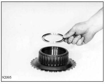
Start adding parts to 1st gear freewheel 77.120 by pressing in one of the two cover plates 77.120/120 for the complete freewheel into freewheel ring F.
