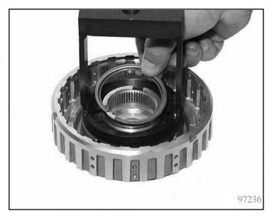
Insert complete disc set C starting with spring disc 75.010/170 followed by outer clutch disc 75.010/180 and lined clutch disc 75.010/190.
