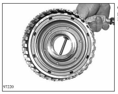
Cover one of the two oil feed bores and press out the piston with compressed air. Pull the three O-rings off piston B.
