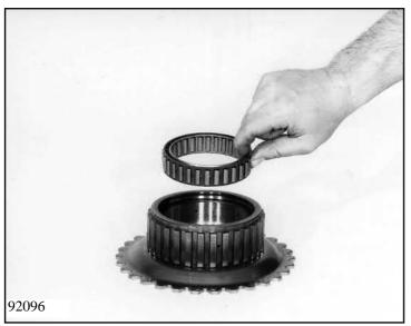
Insert freewheel cage 77.120/120 into the freewheel outer ring with the collar upwards.
