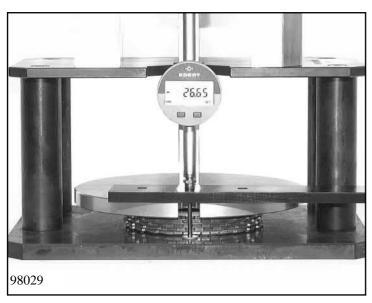
Determine thickness  $M_A$  of the disc set for clutch A as described in Chapter 1.4.0 "Measuring the clutch packs".
