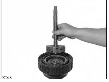
Lift up the intermediate shaft with inner disc carrier A. Remove axial needle bearing.
