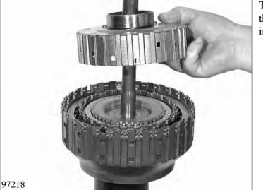
Take out inner disc carrier B and lift off the axial needle roller bearing from the intermediate shaft.
