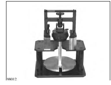
Fasten adjusting device with 4 knurled screws to the measuring fixture using the intermediate pieces. Connect measuring plate 5p01 040 330 to force-measuring unit using fixing pin.
