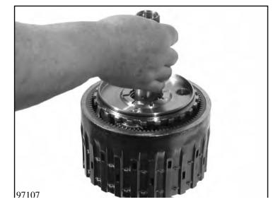
Turn the planetary drive as you put it on the planet carrier.
