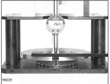
Determine thickness  $M_A$  of the clutch A clutch pack according to Chapter 1.4.0: Measuring the clutch pack.
