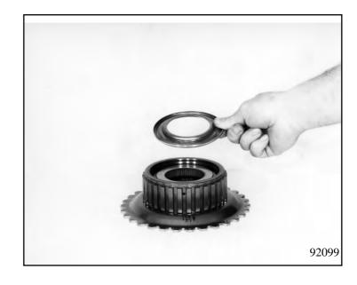
Insert the complete freewheel into brake F, turning it as you put it in. Now insert snap ring 77.130 using assembly tool 5x46 000 892 (or by hand).
