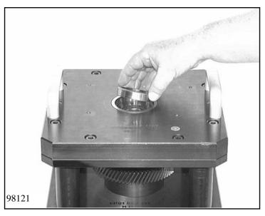
Put outer bearing shell on side shaft and measuring bell 5p01 130 331 on the bearing outer ring.
