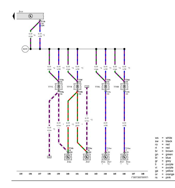
Driver door control unit, Front passenger door control unit, Onboard supply control unit, Rear driver side door control unit, Rear passenger side door control unit
