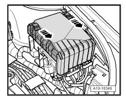
Remove bevel box (manual gearbox) ⇒ Gearbox; Rep. gr. 34.
