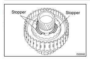
(g) Set the end gap of the snap ring in the underdrive clutch drum shown in the illustration.
