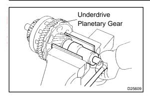
(c) Using a socket wrench, remove the lock nut.
