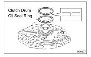
16. INSTALL CLUTCH DRUM OIL SEAL RING
