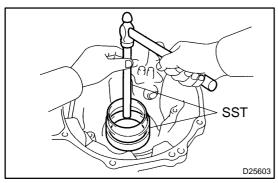
(b) Using SST, install the outer race of the tapered roller bearing FR.
