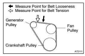
(b) Press the center point of the V belt with a load of approx.98 N (10 kgf, 22 lbf) and adjust the V belt deflection so that it should be within the standard value.
