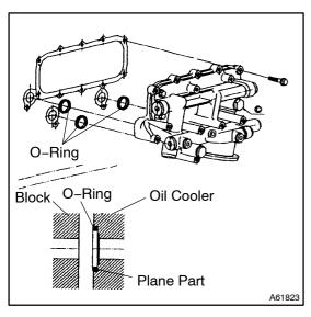
(b) Insert new O-rings into the O-ring groove of the oil cooler. HINT:
