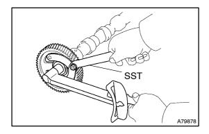
(d) Using SST, install the plate washer and bolt. SST 09960-10010 (09962-01000, 09963-01000) Torque 57 N·m (581 kgf·cm, 42 ft·lbf)
