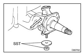
(c) Insert SSTs to the thread of the guide, and turn the nut until the nut begins to fix.
