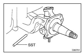
(b) Insert SST to the hole of the lock pin and fix the guide in the I-beam.
