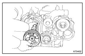
Install the camshaft timing gear or sprocket into the cylinder block.
