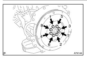
(c) Install the bolts, as shown in the illustration.
