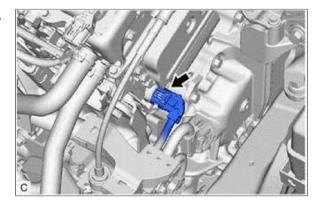
Check the connection condition of the motor temperature sensor connector and the contact pressure of each terminal. Check the terminals for deformation, and check the connector for water ingress and foreign matter. Click hereGeneral>INTRODUCTION>HOW TO TROUBLESHOOT ECU CONTROLLED SYSTEMS>ELECTRONIC CIRCUIT INSPECTION PROCEDURE
