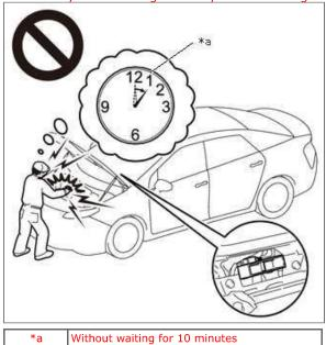
After removing the service plug grip, wait for at least 10 minutes before touching any of the high-voltage connectors or terminals. After waiting for 10 minutes, check the voltage at the terminals in the inspection point in the inverter with converter assembly. The voltage should be 0 V before beginning work.
