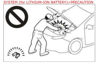
To prevent electric shock, wear insulated gloves when working on wire harnesses and components of the high voltage system.
