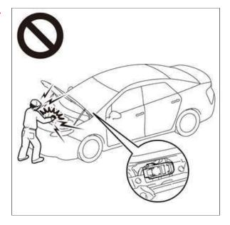
To prevent electric shock, make sure to remove the service plug grip to cut off the high voltage circuit before servicing the vehicle.
