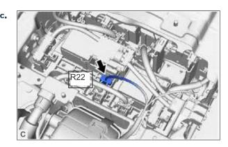
Disconnect the R22 HV battery junction block assembly connector.
