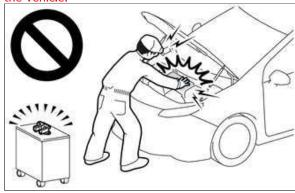
After removing the service plug grip from the HV battery, put it in your pocket to prevent other technicians from accidentally reconnecting it while you are working on the high-voltage system.
