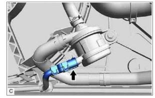
Check the connector connections and contact pressure of the relevant terminals for the inverter water pump assembly connector.
