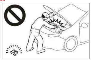
Before the following operations are conducted, take precautions to prevent electric shock by turning the power switch off, wearing insulated gloves, and removing the service plug grip from HV battery.
