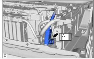
Disconnect the HV battery high voltage connector.
