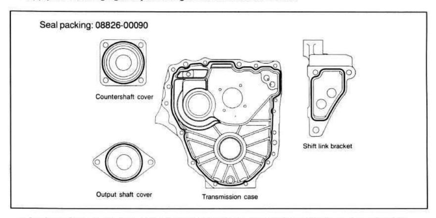
Apply sealing agent also on the threaded portions of set bolts at the time of reassembly.
