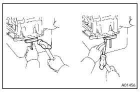
(b) Insert the blade of SST between the bearing cap sub-assembly and oil pan, and cut off applied sealer and remove the oil pan.
