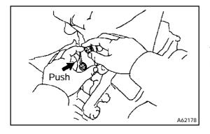
(2) Apply engine oil to the chain tensioner and install it. Torque: 9.0 N·m (92 kgf·cm, 80 in·lbf)
