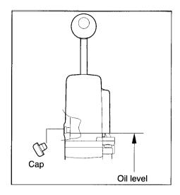
Note that the presence of air in the oil can cause the engine to not tilt up and down properly.
