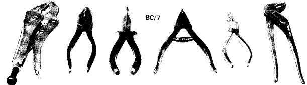
Vice grip pliers, ordinary pliers, long nose pliers, circlip pliers (expanding type), circlip pliers (contracting type) and multigrip pliers.
