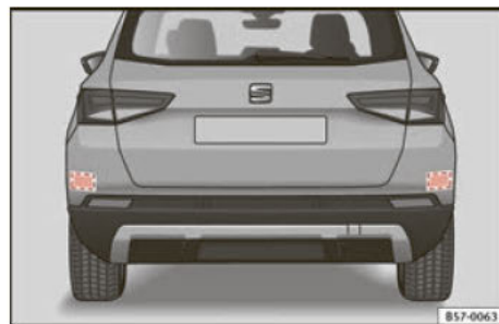
Fig. 193 Rear view of the vehicle: radar sensor zones.
