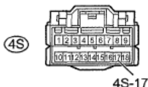
Fig. 40: Identifying F17 Telltale Light And 4S Main Body ECU Connectors Courtesy of TOYOTA MOTOR SALES, U.S.A., INC.
