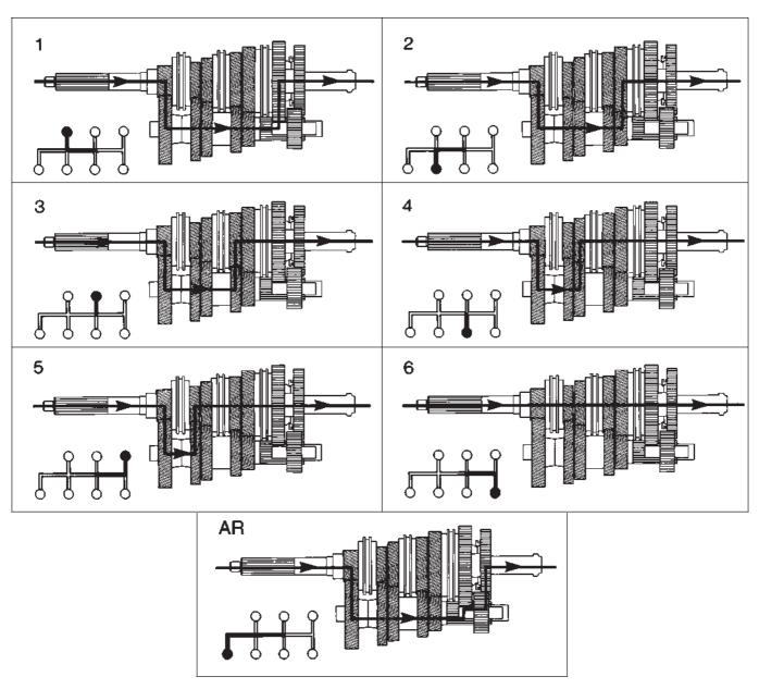
Power flow diagrams - direct drive top gear version
