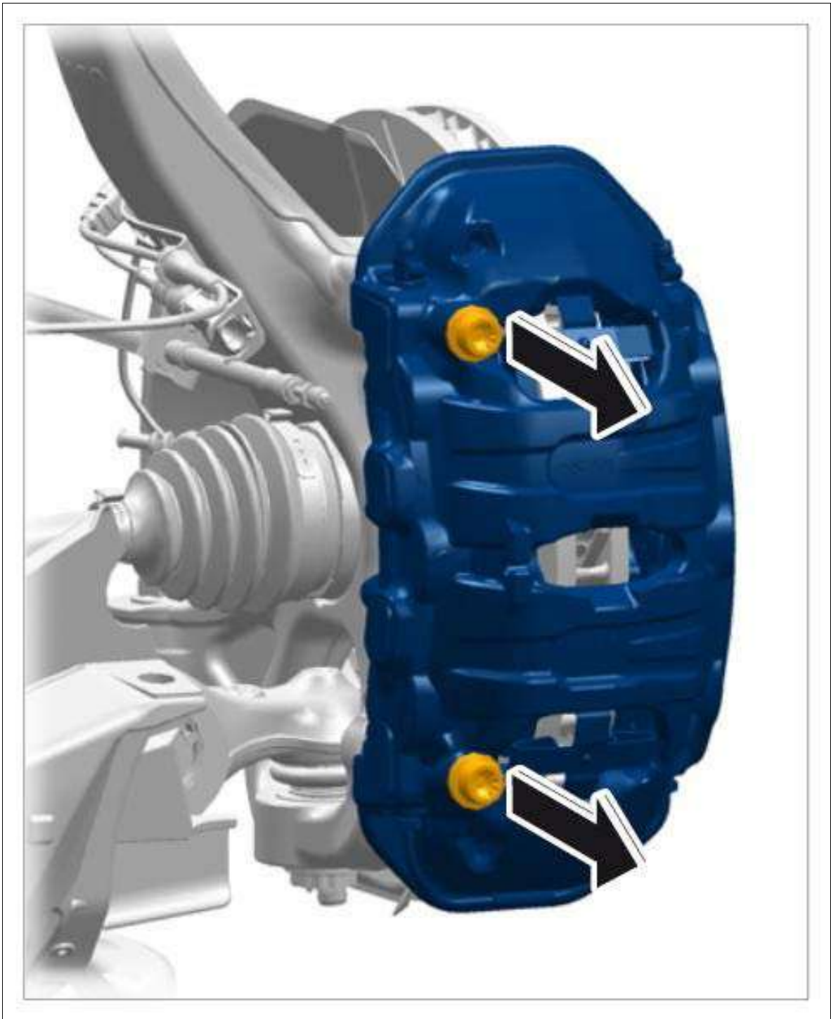
Fig 7: Removing Brake Caliper Fastening Screws
