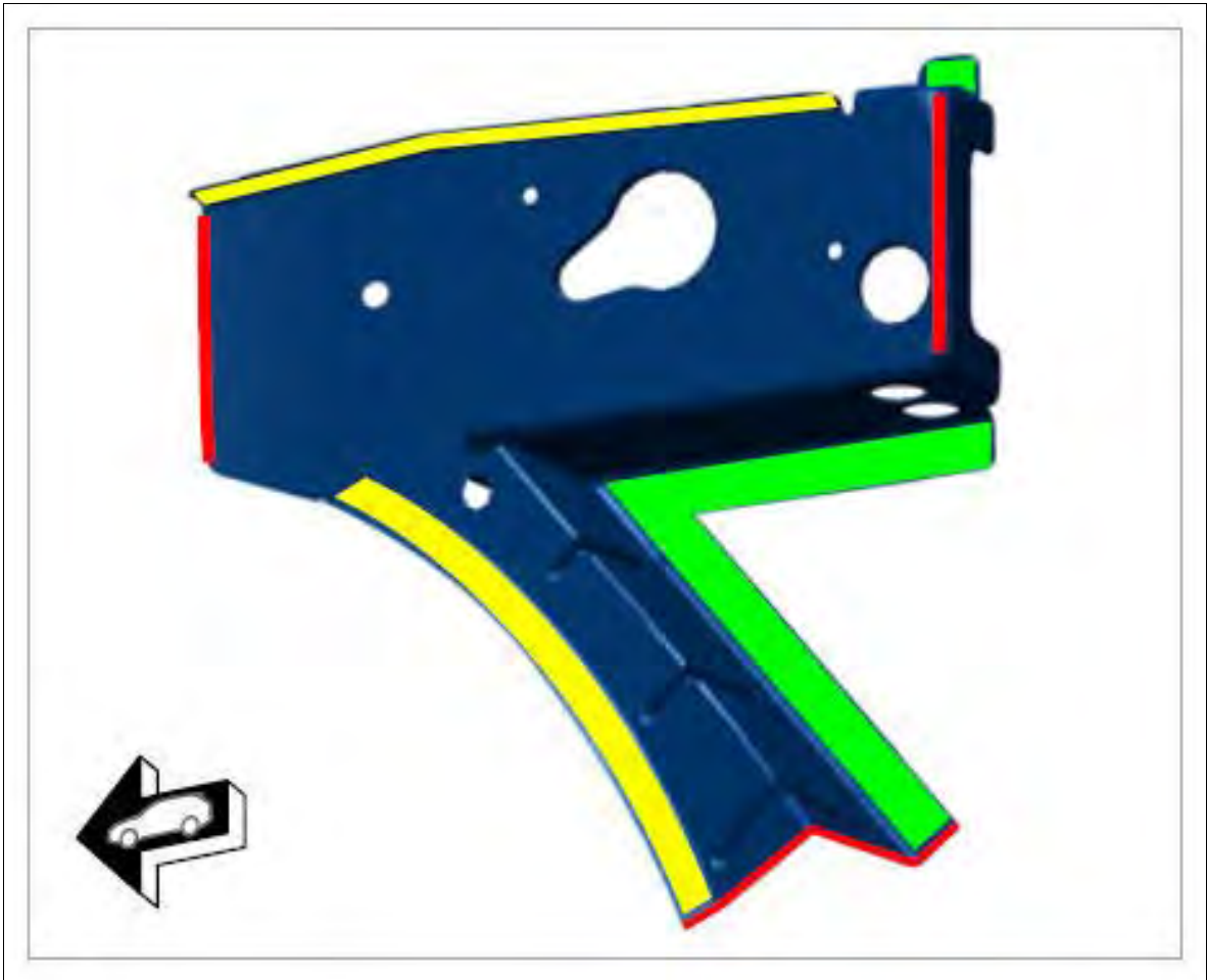
Fig 5: Removing Reinforcement For Bonding
