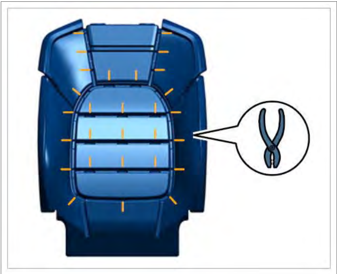
Fig 2: Detaching Front Backrest Padding From Cover (Sport)
