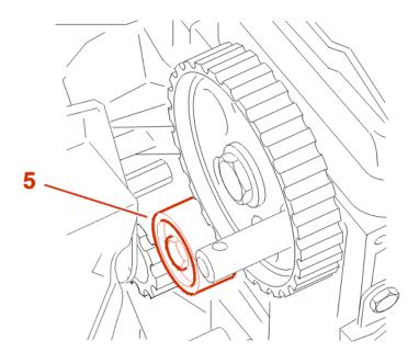
Check that the roller tensioner (5) turns freely (no tight spot).
