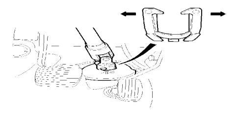
Release the steering universal joint by moving aside the safety clip.
