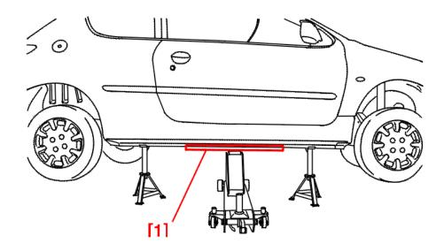
Position the axle stand in the location provided for lifting the vehicle using the jack.
