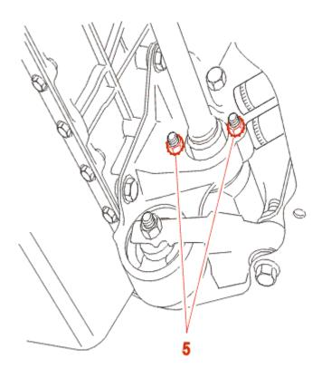
Pre-tighten one bearing nut (5) to 0.5 daN.m.
