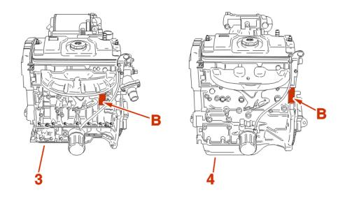
(3)Engine : Aluminium cylinder block .
