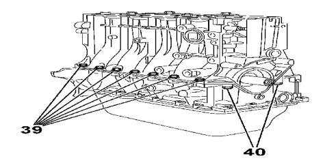
Remove all of the securing bolts (39) and (40) from the main bearing cap casting.
