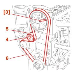
Slacken the nut (4) retaining the roller tensioner (5) to slacken the belt (6).
