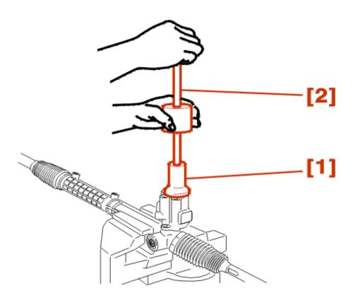
Fit the distributor valve (7) using the tools [1], [2].
