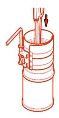
Position the piston on the liner to obtain on fitting:
