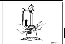
c. If not within specification, adjust clearance by changing thickness of differential side gear thrust washers.
