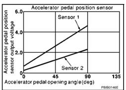
Idle position of the accelerator pedal is determined by the ECM
