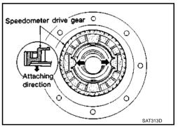
6. Install final gear and tighten fixing bolts in a numerical order.
