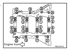
ii. Turn M10 bolts  $90^{\circ}$  clockwise in numerical order from No. 1 to 16 using Tool.
