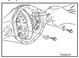
c. Tighten or loosen each side bearing adjuster using Tool.
