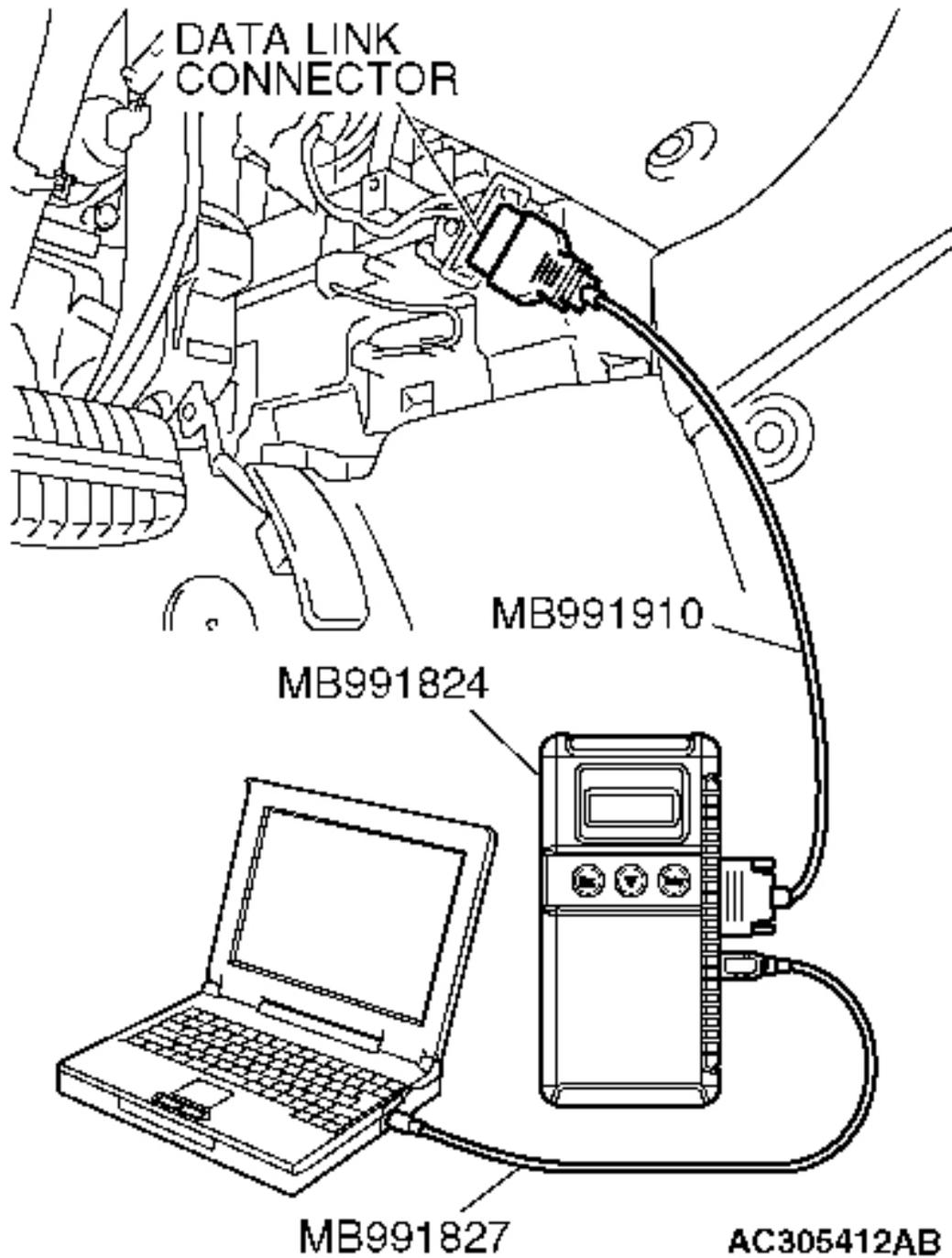
**Fig. 627: Connecting Scan Tool To Data Link Connector**
