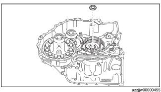
6. Remove the pinion shaft.
