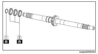
20. Remove the thrust needle bearing.
