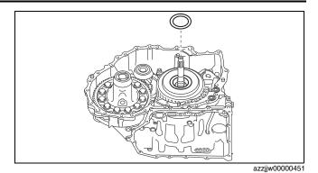
17. Remove the clutch component.
