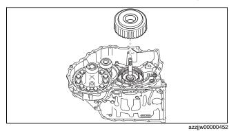
18. Remove the turbine shaft.
