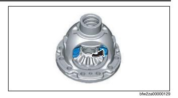
5. Assemble the pinion shaft.
