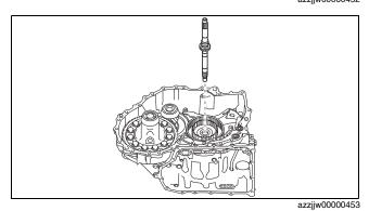
19. Remove the D-ring and seal rings from the turbine shaft using the procedure in the figure:
