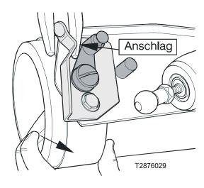
Gap with the operating cylinder detached and the exhaust brake flap closed by hand.
