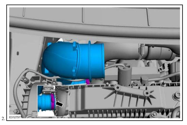
1. Install the air cleaner outlet pipe and tighten the clamp.
