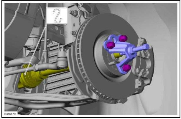
8. Remove and discard the halfshaft retaining strap and nuts.
