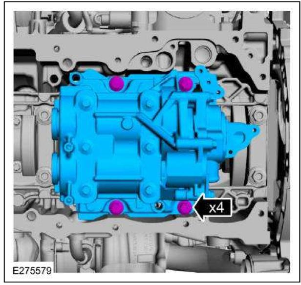
6. Tighten the bolts in sequence shown.
