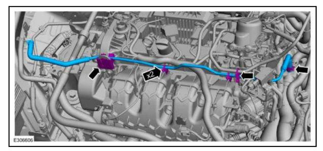
93. Position the ground wire, attach the retainer and install the bolt.
