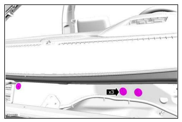
14. Release the clips and remove the LH trim panel.
