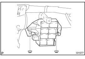
(c) Install the steering side connector block with the 2 nuts.
