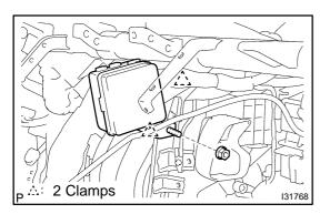
Install the passenger side junction block with the nut and (c) 2 clamps.
