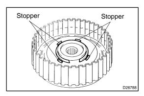
(g) Set the end gap of the snap ring in the piston shown in the illustration.
