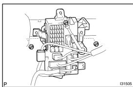
(d) Install the driver side junction block with the 3 nuts. Torque: 8.4 N·m (85 kgf·cm, 73 in. lbf)
