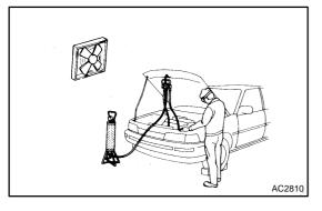
DO NOT HANDLE REFRIGERANT IN AN ENCLOSED AREA OR NEAR AN OPEN FLAME
