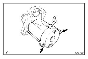
(b) Install the starter field frame with the 2 through bolts. **Torque: 6.0 N·m (61 kgf·cm, 53 in.·lbf)**
