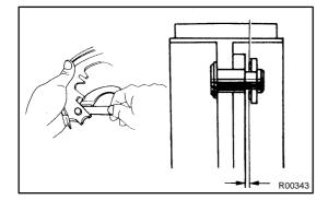
(b) Using a feeler gauge, measure the clearance. Standard clearance: Less than 0.35 mm (0.0138 in.) If the clearance is not within the specification, replace the shim with one of the correct size.
