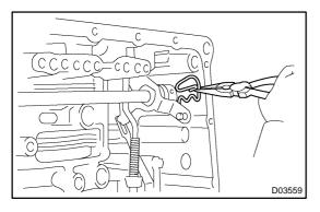
21. REMOVE B-3 ACCUMULATOR PISTON
