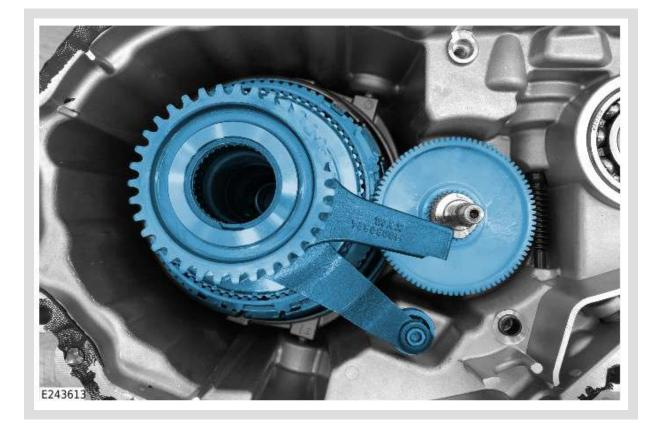
Remove the transfer differential assembly.
