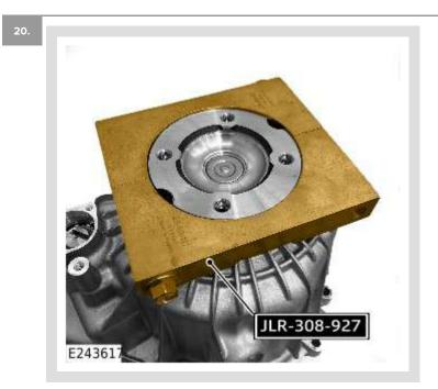
Install the special tool. Install the Special Tool(s): JLR-308-927
