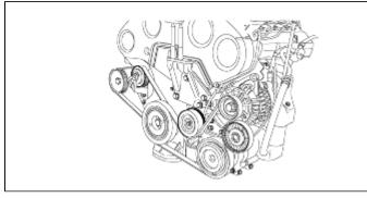
3. After installing the belt loosening the adjustment bolt counter clockwise at the "Q" arrow indication, apply tension to the belt by tightening the bolt clockwise.
