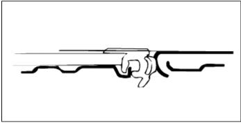
(1) Loosen the front screw and rear screw and adjust the height between the glass panel and roof panel.
