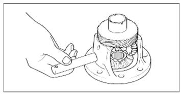
(4) Check the side gear pinion backlash and install a proper spacer.
