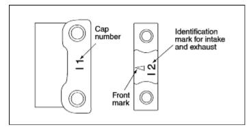
6. Tighten the bearing cap in two or three steps. Tighten it to the standard torque at the last stage. \*Bearing cap standard torque
