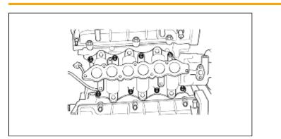
2. Install the delivery pipe and injector assembly to the intake manifold.
