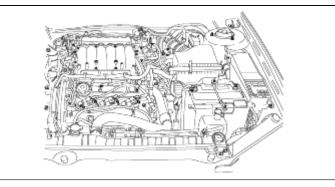
2. Remove the engine wiring and the transaxle wiring.
