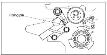
2. How to check tension (While auto tensioner is operating : and fixing pin being uninstalled.)
