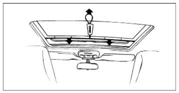
(6) After adjustment, be sure to sure to lock the nut with the pawl washer.
