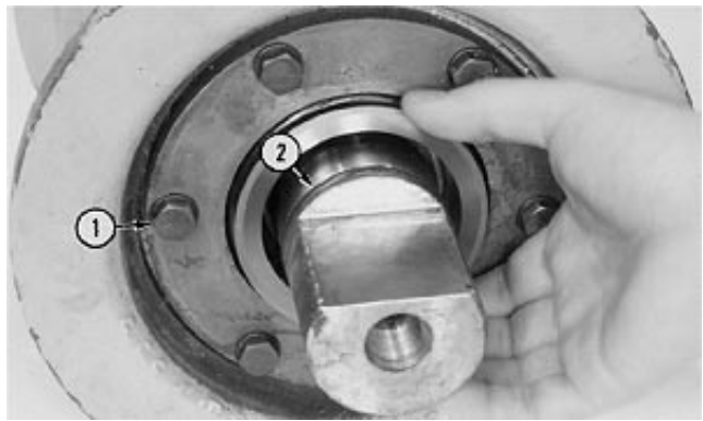
1—Cap Screw (12 used) 2—O-Rings
