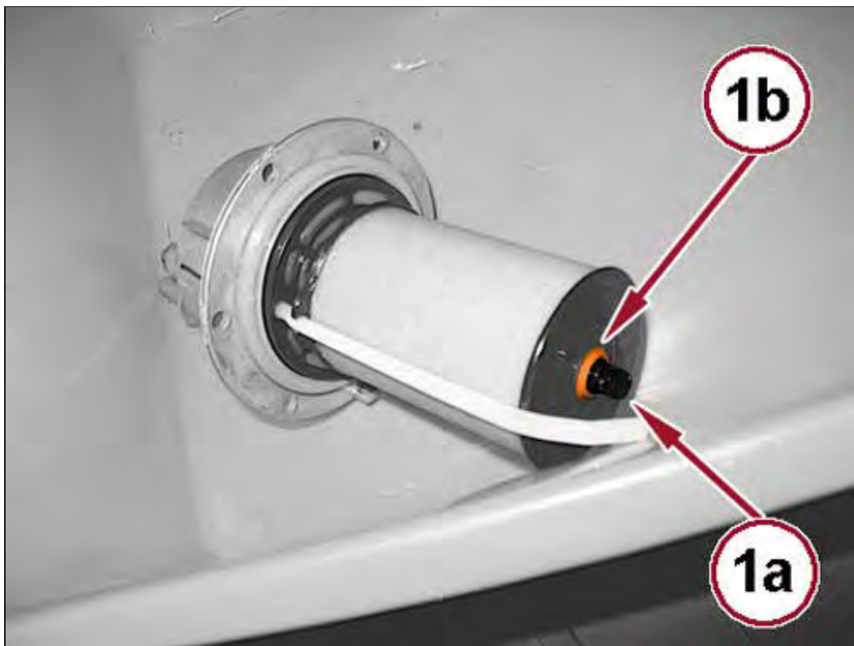
Fig 8: Water Presence Sensor & Seal Ring
