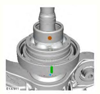
CAUTION: Using the 3mm drill mark and paint mark on the differential drive pinion flange damper and paint alignment mark on the driveshaft (as indicated). Make sure that the alignment marks are correctly aligned.
