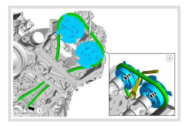
Install the timing chain with the VVT units.
