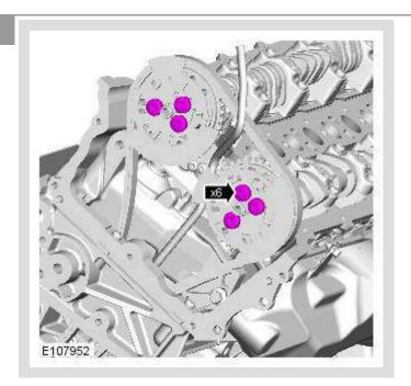
Install the variable valve timing (VVT) unit bolts finger tight at this stage.
