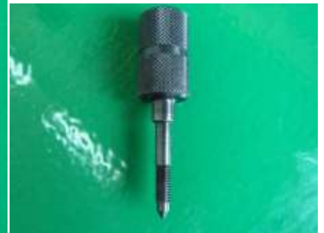
Valve Installing Locating Needle
