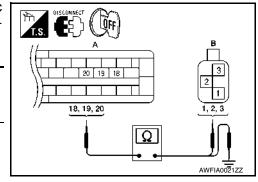
Measure the continuity between the ABS actuator and electric unit (control unit) harness connector E125
