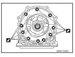
58. Tighten oil pump bolts ( to the specified torque.
