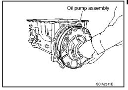
57. Apply recommended sealant to oil pump assembly as shown in the figure.
