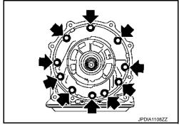
59. Install O-ring to input clutch assembly.
