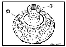
56. Install oil pump assembly (with under drive sun gear) to transmission case.
