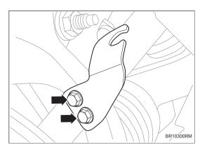
(f) Remove 2 bolts to detach the front brake hose bracket.
