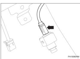
(b) Connect the front camera assembly harness connector.
