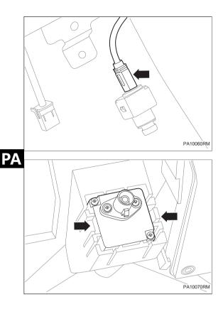
(a) Disconnect the front camera assembly harness connector.
