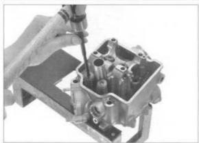
Install the insulator to the cylinder head by aligning the groove of the insulator with the tab of the cylinder head.
