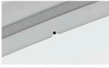
D, H Outer Panel Roof Opening Flange Notch (4 places)
