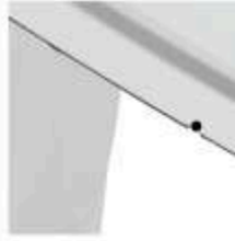
F, J Outer Panel Door Opening Flange Notch (4 places)
