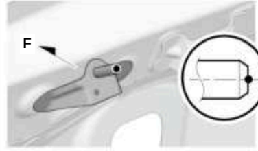
D, H Outer Panel Roof Opening Flange Notch (4 places)
