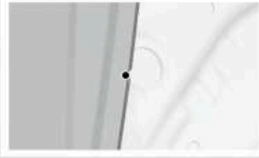
E, e, G, g, I, K, k Outer Panel Door Opening Flange Notch (8 places)
