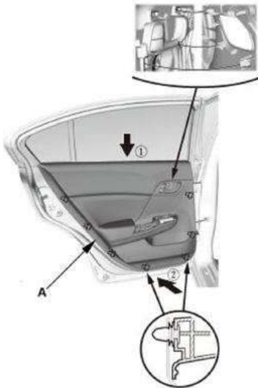
Fig. 550: Installing Rear Door Panel Courtesy of AMERICAN HONDA MOTOR CO., INC.
